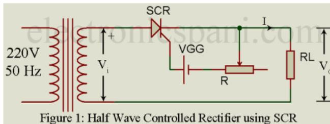
Figure 1: Half Wave Controlled Rectifier using SCR
