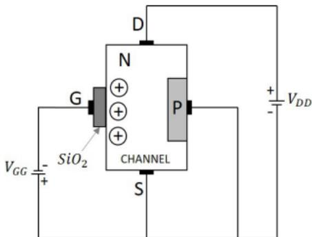
Working of MOSFET in depletion mode
