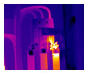
Fig 1. The Thermal Image of electrical connector
