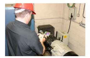
Fig 2. The inspection of electrical equipment using a Thermal Imager
