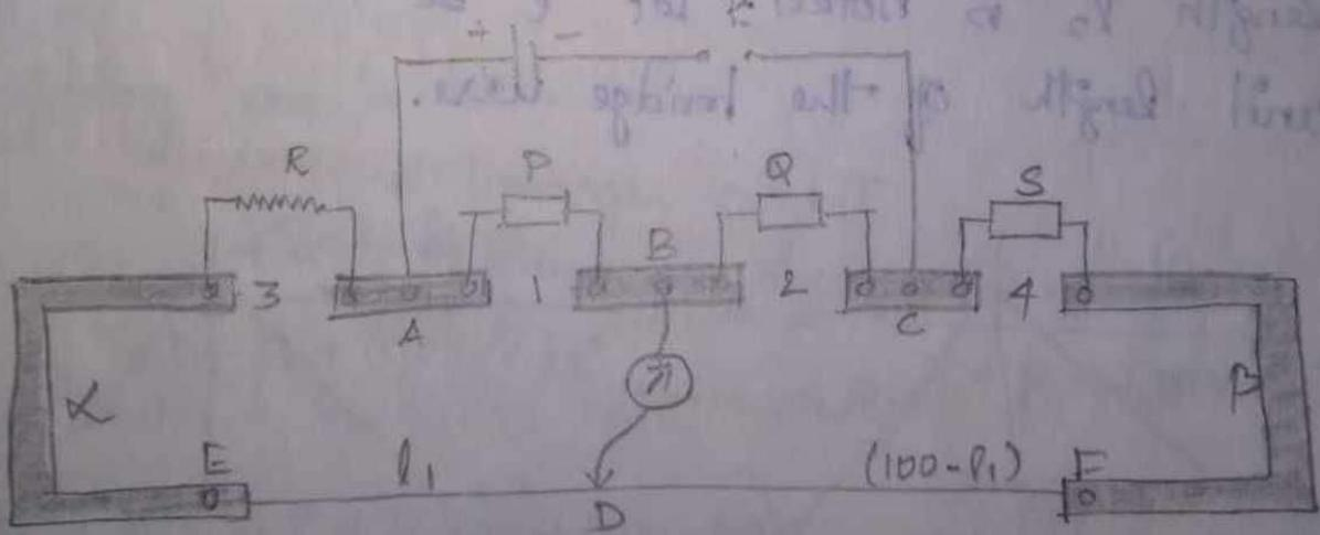
P and Q are two resistance boxes connected in the inner gaps 1 and 2, R is the unknown low resistance and S is a fractional resistance box.
