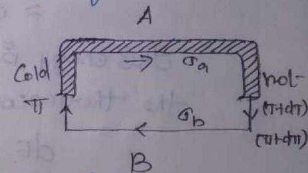
Heat energy absorbed due to Peltier effect at
