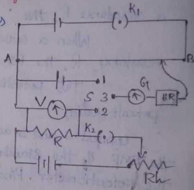
The balancing length  $l$  for the standard cell is determined first.
