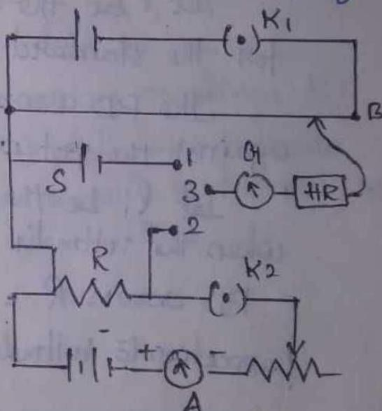
11) , the corrections for other ammeter readings are determined. A Calibration curve is plotted for ammeter, taking ammeter readings on X-axis and correction on Y-axis.
