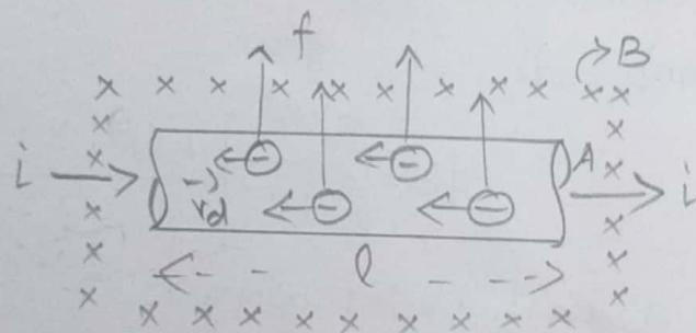
The electric current  $i$  in a conductor is due to free electrons moving in a direction opposite to the direction of the electric current.
