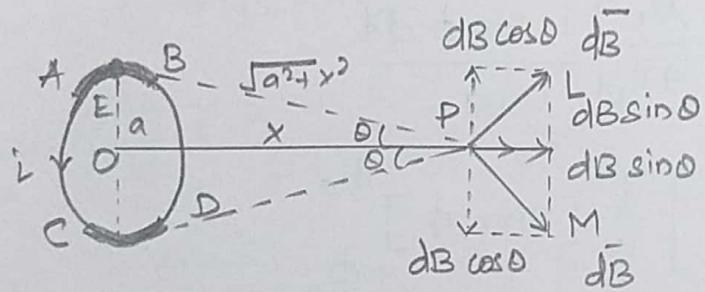
$$\text{The field at } P \text{ due to } AB = dB = \left[ \frac{\mu_0}{4\pi} \right] \frac{i dl}{(a^2 + x^2)}$$
