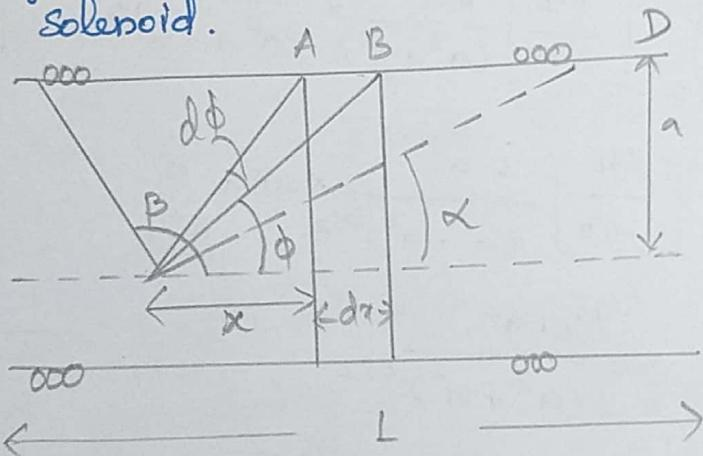
Consider an elementary length  $dx$  of the solenoid, at a distance  $x$  from  $P$ .
