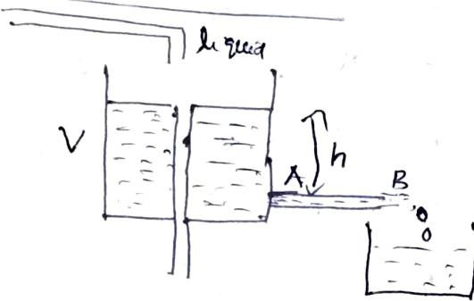
The liquid is taken in the constant level tank up to a height  $h$ . A capillary tube AB is fixed at the bottom of the ~~tank~~
