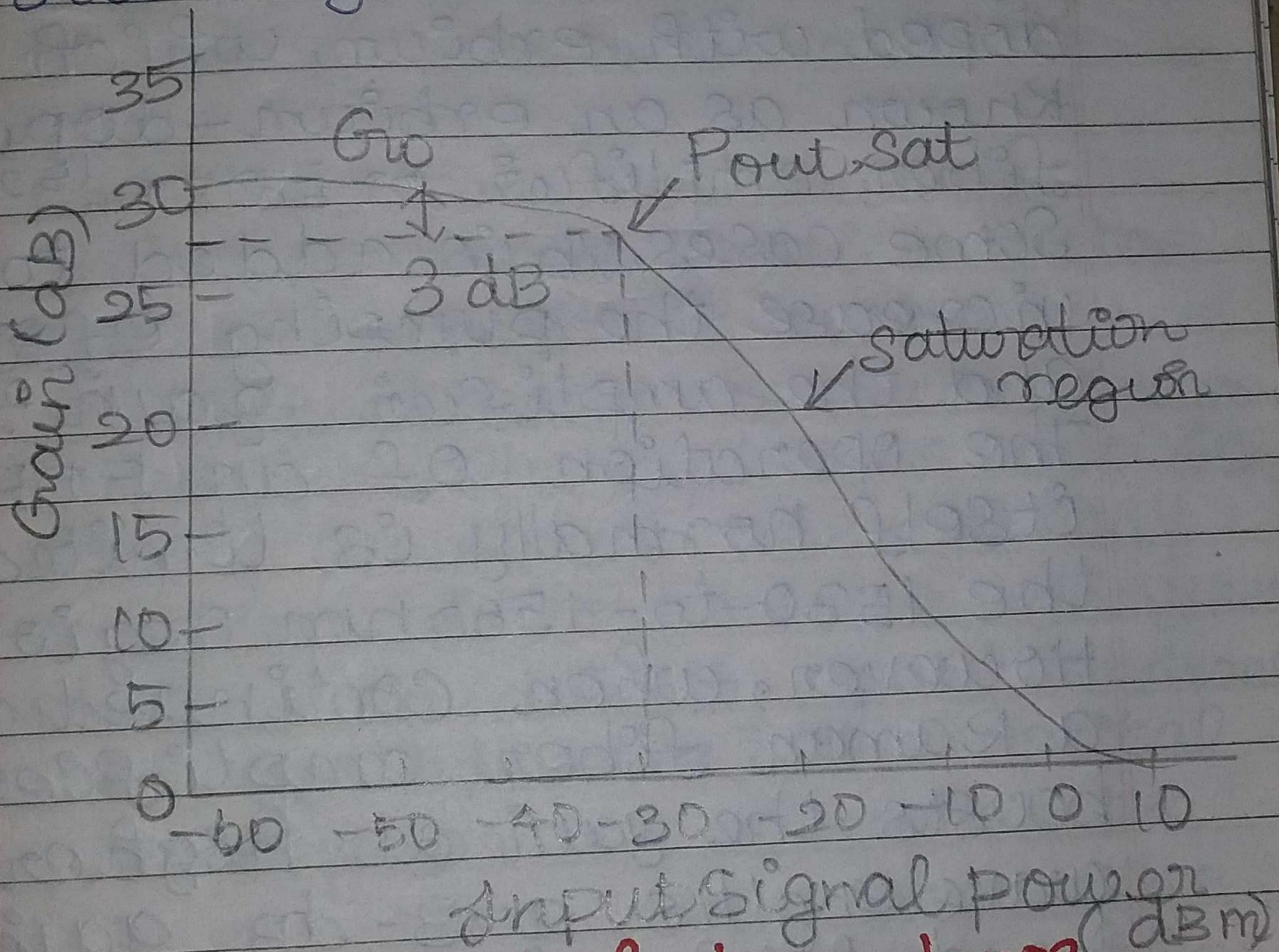
Typical dependence of the single pass-gain on optical input power for a small signal gain of  $G_0=3 \text{ dB}$  (a gain of 1000).
